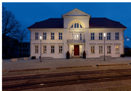
10 Deviating from the standard version, for this project small FLC121 projectors have been integrated into the PMMA cylinders. As a result, both the path lighting and the architectural lighting are produced from a single luminaire.
